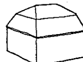
dual-pitched, hipped ("mansard" when steep lower slope)
